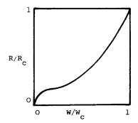
Fig. 1 Dimensionless drying curves - porous granules.
